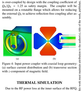
Figure 4: Input power coupler with coaxial loop geometry: (a) surface current distribution and (b) transverse section with z-component of magnetic field.
