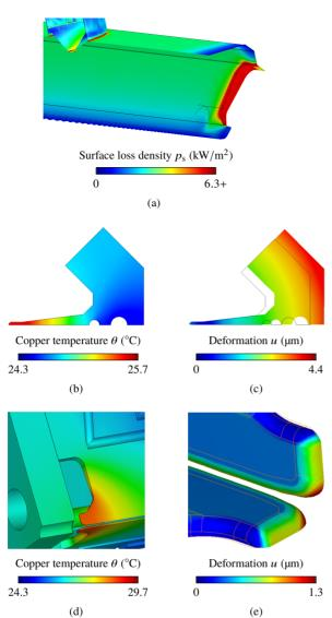
licence (© 2018). Any distribution of this work must maintain attribution to the author(s), title of the work, publisher, and DOI. Figure 5: Thermal simulation results for nominal parameters (2.5 % duty cycle,  $\theta_{\rm w} = 22$  °C,  $v_{\rm w} = 1$  m/s). (a) Power loss  $p_s$  on cavity surface. (b) temperature  $\theta$  and (c) deformation u of the octant-symmetric cross section; (d), (e) respective results around the vane nose.
