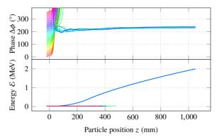
Figure 7: Phase and energy of the tracked particles along the RFO. The color indicates the start phase of the particle relative to the RF field.
