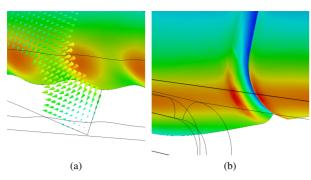
Figure 2: Surface and transverse electric field (a) at the vane and (b) at the module gap with a maximum of  $E_{\rm s} = 39.1 \, {\rm MV/m}$ .
