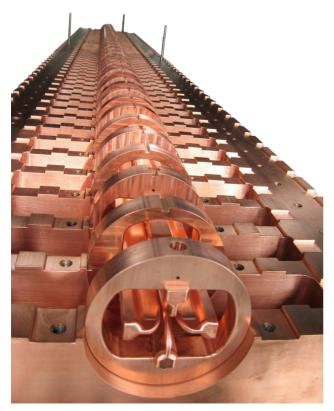
Figure 3: Assembly of the electrodes and carrier rings.
