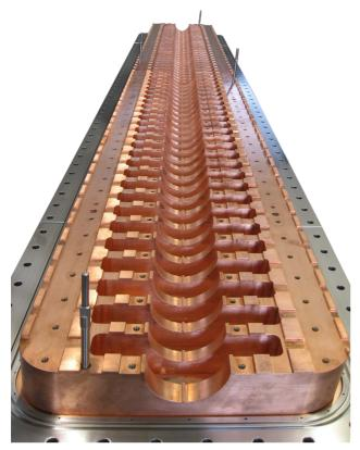
Figure 2: Lower half-ladder structure after finalization of surface treatment and assembly on the lower tank shell.
