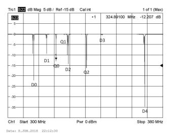
Figure 6: Frequency spectrum of XiPAF RFQ after final tuning (22 °C, 10% humidity).
