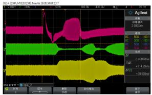
Figure 1: The signal with pickup-drop on oscilloscope.
