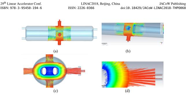
Figure 4: The FE particles trajectory simulation of HWR.
