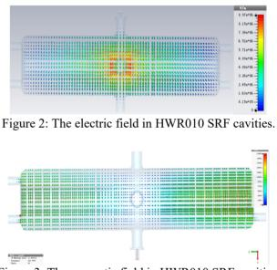
Figure 3: The magnetic field in HWR010 SRF cavities.
