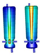
Figure 1: Magnetic field distribution (left) and electric field distribution (right) for the 81.25 MHz mode.
