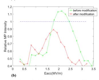
Figure 4: Top shorting plate modification (a) relative MP Intensity before and after modification (b).
