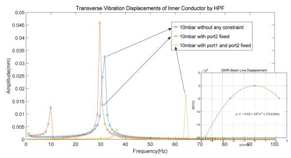
Figure 3: Transverse frequency response of drift tube to HPF.
