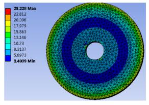
Figure 6: Thermal stress on the ceramic surface.
