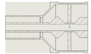
Figure 2: Schematic drawing of CEPC klystron output window.
