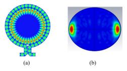
Figure 2: Top-view and side-view of "Whispering Gallery" mode.
