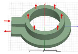
Figure 8: Mode launcher of TM<sub>9,1,16</sub>.
