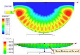
Figure 6: Field distribution inside the cavity and on the wall for  $TM_{9,1,16}$  mode.
