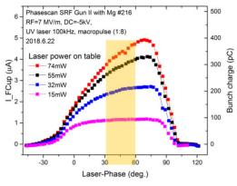
Figure 2: Measured Faraday cup current (and bunch charge) vs. drive laser phase. The working laser phase of the SRF gun is indicated by the vertical zone ( $40^{\circ}$  to  $60^{\circ}$ ).
