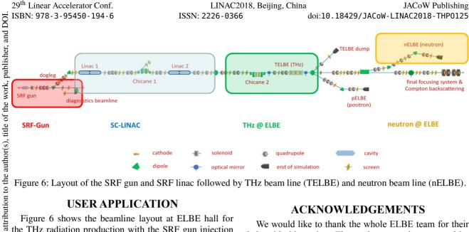
Figure 6: Layout of the SRF gun and SRF linac followed by THz beam line (TELBE) and neutron beam line (nELBE).
