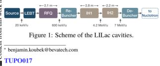
The Linac consists of 5 cavities, an RFQ followed by a rebuncher, 2 IH-DTL structures and a de-buncher as shown in Fig. 1. It is operating at 162.5 MHz with a beam repetition rate of 5 Hz and a duty cycle of 0.15% [2]. The main parameters of the LILac are summarised in Table 1. The length of the Linac comprising the cavities, the beam diagnostic devices and focusing magnets but excluding the de-buncher will be realised within a length of 9 m. A scheme of the LILac cavities is shown in Table1.
