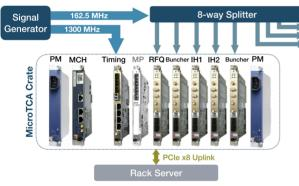
BY 3.0 licence (© 2018). Any distribution of this Figure 4: Layout of the LLRF system including RF master oscillator, LLRF controller channels and CPU processing 20 unit.
