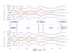
Figure 2: Transverse beam envelopes of the LILac DTL section, 15 mA, A/q = 3.
