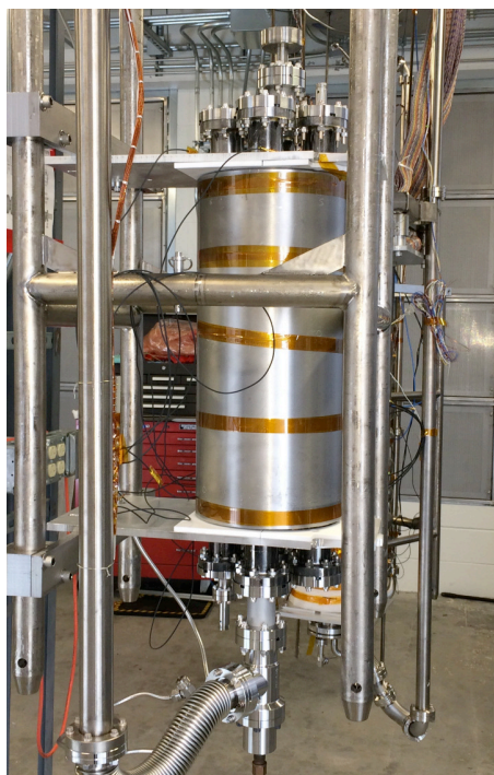
Figure 3: Assembled cavity taken out from clean room.
