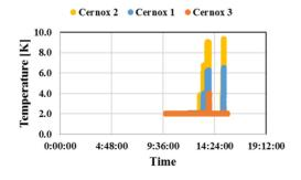
may Figure 9: Measured temperature change in Cernox sensors.
