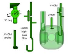
Figure 4: HHOM and VHOM couplers for the rf-dipole crabbing cavity.
