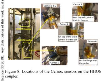
Figure 8: Locations of the Cernox sensors on the HHOM coupler.
