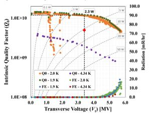
Figure 3: Q curves of the bare RFD-CAV-002.
