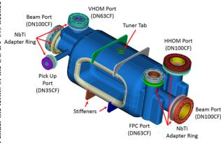
Figure 1: 400 MHz SPS prototype rf-dipole cavity.
