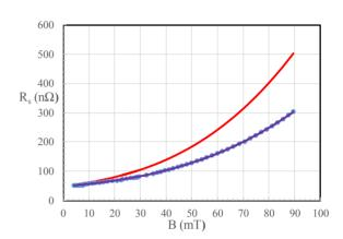
Figure 5: Average surface resistance (blue dots), polynomial fit (purple curve) and derived actual surface resistance (red curve) from the Q-curve of Fig. 4.
