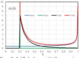
Figure 2: da/dh for the coaxial half-wave cavity.
