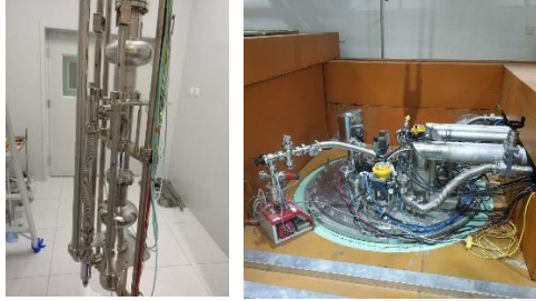
Figure 3a: Two single cell cavities were assembled together. 3b: Vertical test system at Peking University.
