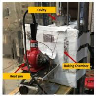
Figure 3: Set-up of 75C baking on the wave-guide insert.
