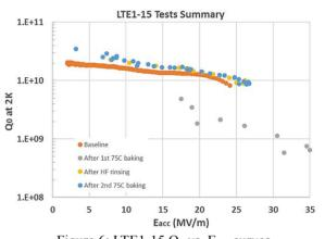
Figure 6: LTE1-15  $Q_0$  vs.  $E_{acc}$  curves.
