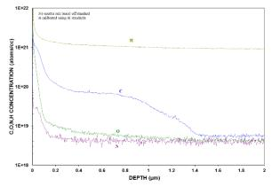
(b) SIMS data of samples baked at 120°C under N<sub>2</sub>. Figure 2: SIMS data comparison between 120°C baking under vacuum and under N<sub>2</sub>.
