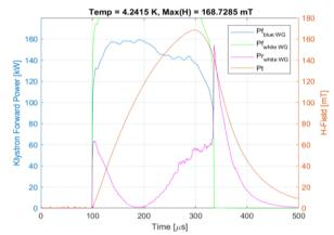
Figure 5: HPP test results after 120°C infusion showing the maximum B-field achieved was 169 mT, i.e.  $E_{acc} \sim 40 \text{ MV/m}$ .
