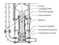
Figure 1: Schematic of wave-guide insert allowing regular CW and high-power pulse measurement in same cryogenic cvcle.
