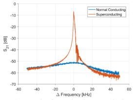
Figure 2: Example of normal and superconducting states on the network analyzer.
