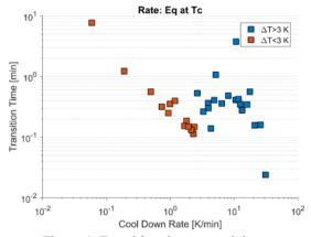
Figure 4: Transition time vs cool down rate.
