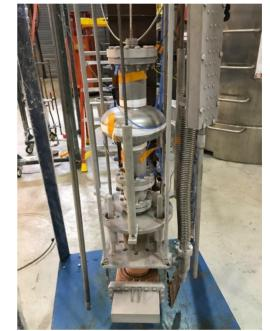
Figure 1: Test insert with single-cell cavity and instrumentation.
