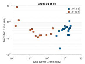
Figure 5: Transition time vs spatial cool down gradient across the cavity cell.
