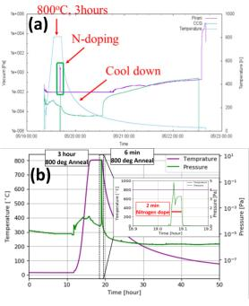
Figure 2: The temperature and pressure data in the nitrogen doping for a) single-cell applied heavy dope [3] and b) threecell applied light dope.
