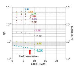
Figure 5: The quality factor measurement retried at each temperature from 1.5 K to 4.2 K.
