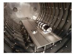
Figure 1: The set-up of nitrogen doping using oil-free furnace at J-PARC.
