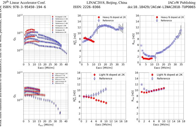
Figure 4: Upper figure shows the result of the heavy doped single-cell cavity. Lower figure shows the result of the light doped three-cell cavity.
