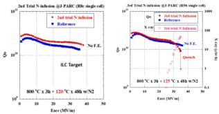
Figure 5: Vertical test results for (left) 2<sup>nd</sup> N-infusion and (right) 3<sup>rd</sup> N-infusion.
