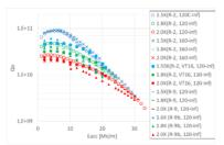
Figure 7: Vertical test results for failed N-infusion.  $1^{st}$ ,  $4^{th}$ ,  $5^{th}$  (R-9) and  $6^{th}$  (R-2&R-9b) N-infusion results are plotted.
