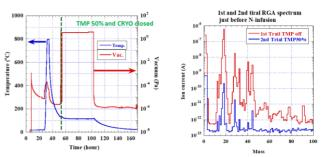
Figure 4: (left) Temperature and vacuum history of typical N-infusion. (right) RGA spectrum of background condition during N-injection. Data was taken without Nitrogen.
