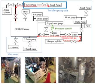
Figure 2: (top) Diagram for N-injection system. (leftbottom) TMPs and scroll pumps. (center-bottom) Portable pumping unit. (right-bottom) N-injection line.
