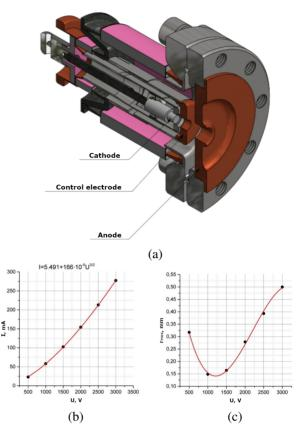
Figure 2: (a) Design of the electron gun of the accelerator for KLT6. (b) Beam current. (c) RMS radius at the enterence to the accelerating structure as function of the control electrode voltage.
