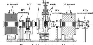
Figure 1: Linac4 test-stand layout.
