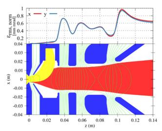
Figure 4: Schematic and emittance evolution of the Linac4's IS03 extraction system at 50 mA beam intensity and an electron to ion ratio of 20. The voltages on the electrodes are (starting from the left) -45kV, -35kV,0,30kV,0.
