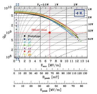
Figure 5: Cavity performance validation. The  $Q_0$  values of bulk cavities measured at 4.2 K are plotted as a function of Eace, Epeak, and Bpeak. Dashed lines indicate lines of constant power dissipation.
