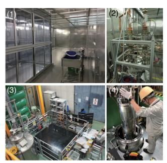
Figure 4: Photos of SRF infrastructure: (1) ISO Class 1 horizontal-flow clean room looking downstream, (2) Coupler test stand in clean room, (3) View of vertical test booth, and (4) Installation of bulk superconducting cavity into the test cryostat for vertical testing (VT).
