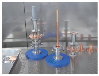
Figure 7: Photo of fundamental power couplers.
