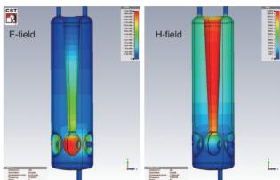
Figure 2: Contour plots of electric (E) and magnetic (H) fields in SC cavity.
