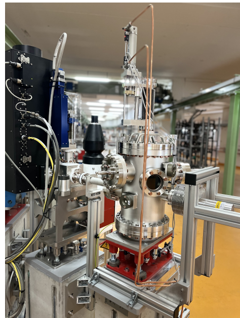
Figure 3: Second experimental area chamber in the dispersive arm of the spectrometer section at the end of the linac. This station is mainly used for detector development with variable pressure inside the chamber.
