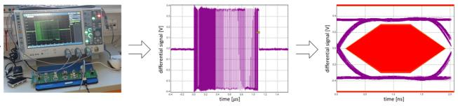
Figure 2: USB signal measurement setup, recorded bit test sequence and the corresponding eye diagram.
