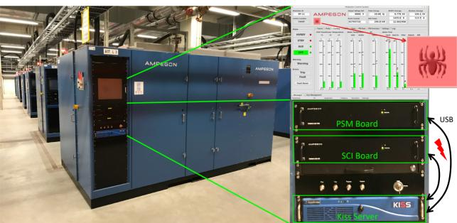
Figure 1: High voltage modulator, GUI and control system.
