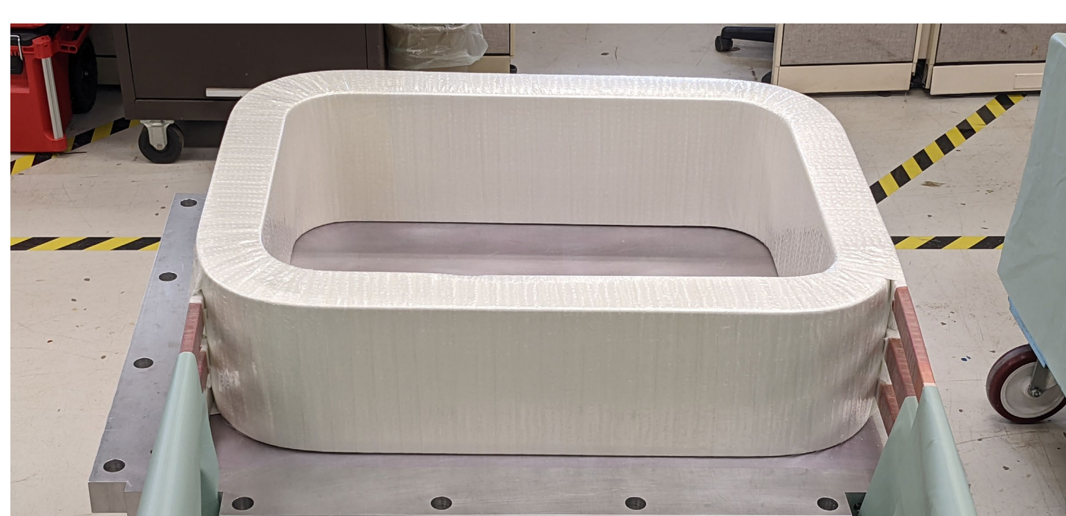
The first chicane magnet coil package insulated and ready for epoxy potting.
