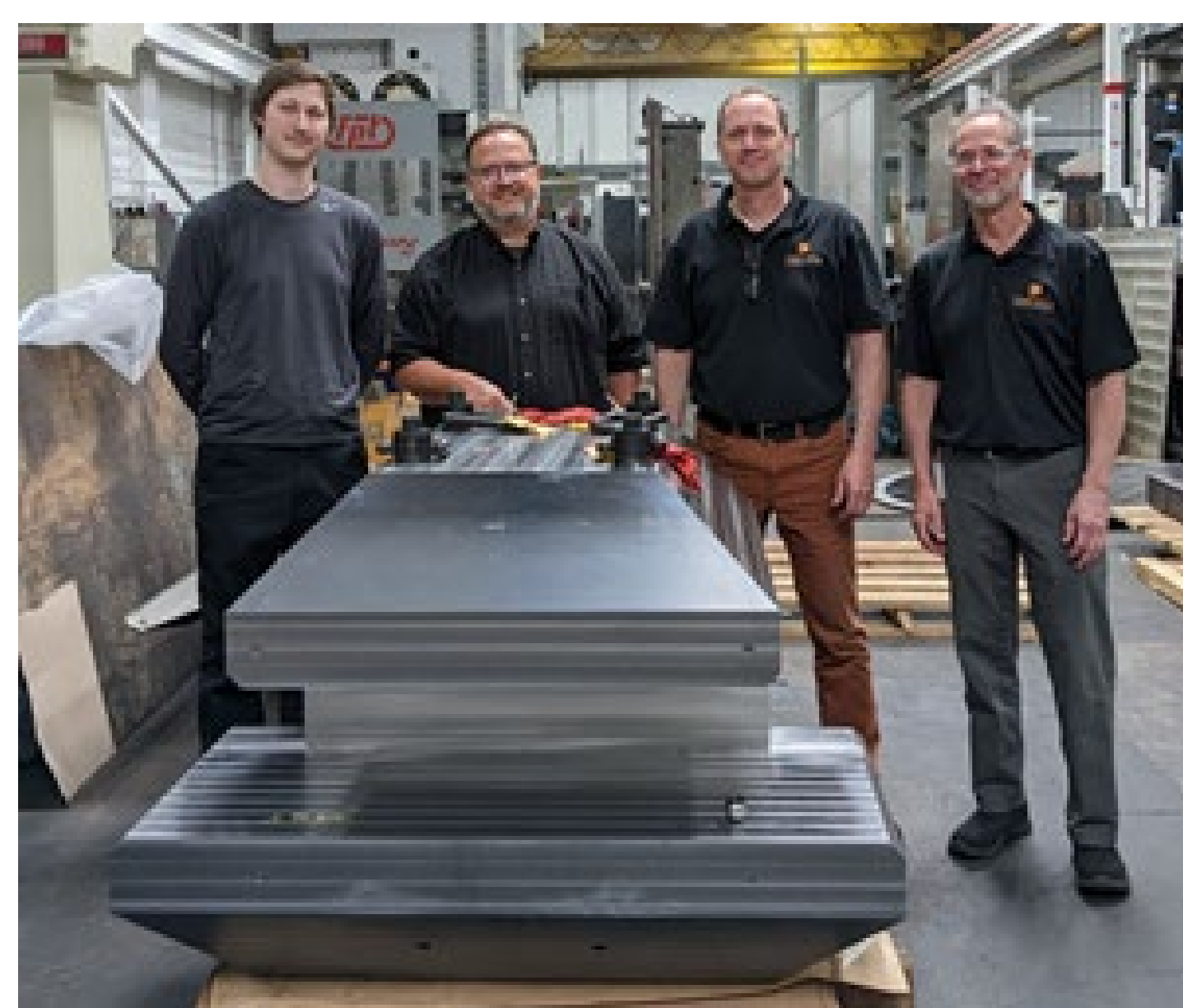
The first chicane magnet core at the vendor
