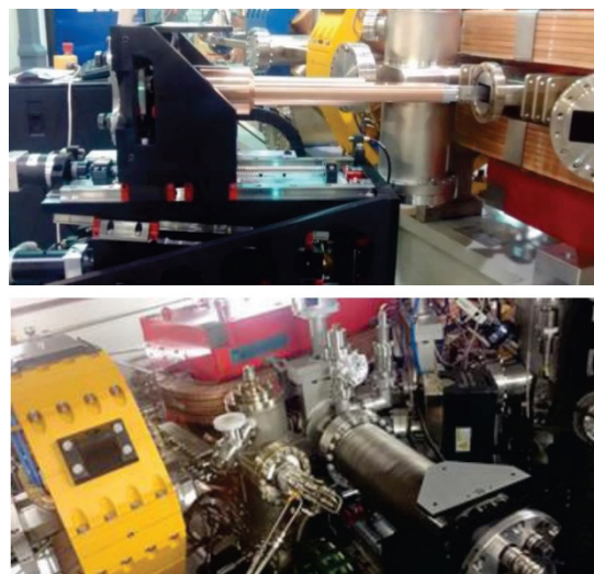
Figure 6: Top: Mechanics assembly mounted on mock-up girder. Down: Extraction mirror retracted mounted inside accelerator's tunnel.
