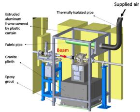
Figure 1: Schematic 3-D drawing of secondary source slits.
