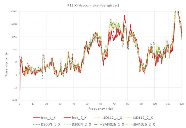
Figure 5: The transmissibility spectrum of R13 in X direction.
