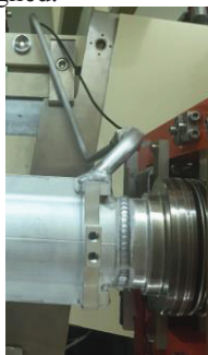
Figure 1: cooling pipe of vacuum chamber.
