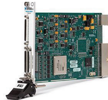
Figure 5: The picture of FPGA Module.
