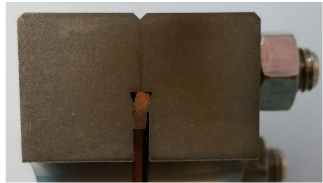
Figure 15: This picture show a gasket can be twist during assembling.
