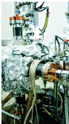
Figure 8: CuCrZr slits in TPS front end 24.
