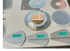
Figure 6: Sample holders and alignment tool.
