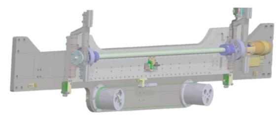
Figure 12: Beamstop actuator.
