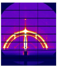
Figure 11: GISAXS image showing beam stop shadows.
