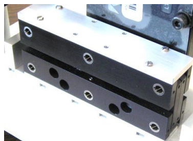
Figure 3: Photograph of the basic deformation compensated linear guiding mechanism for T8-54 linear flexural stage. A total of 12 C-Flex™ D-20 flexural pivots are applied in the linear guiding mechanism.
