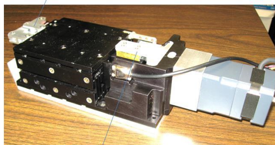
Figure 11: Photograph of the updated compact linear flexure stage T8-54A. The MicroE™ M3500si grating encoder will be replaced by MII6850 grating encoder with reduced interpreter errors.
