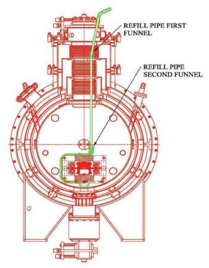
Figure 2 BMIT's wiggler initial refill path.
