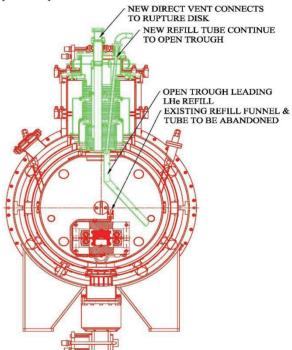
Figure 3 A new vent path & refill path.
