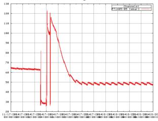
Figure 5 pressure change at LHe transfer line removed.
