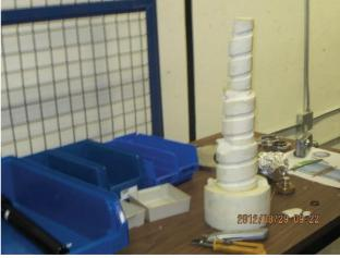
Figure 1 Spiral vent path cut in the insulation foam.
