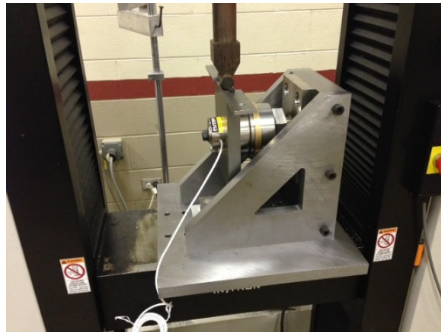
Figure 6: A post-type support installed in an Instron testing machine for lateral stiffness testing.
