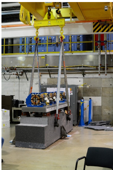
Figure 8: Setup for the free boundary condition, EMA conducted on the ~10000 kg APS-U magnet support prototype. The whole assembly was hung from an overhead crane. The support dynamics were sufficiently lower in frequency than the structural dynamics such that they did not confound the identification of these dynamics.
