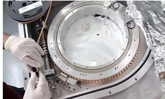
Figure 6: Vacuum cleaning procedures during assembly.
