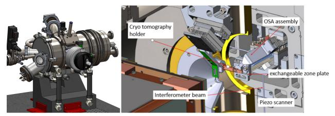
Figure 1: CAD models of the Nanosurveyor 2 instrument showing Gatan cryo tomography sample holder and internal zone plate optic scanning hardware with reference to TEM sample holder.
