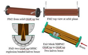
Figure 2: Three styles of masks in HHLFE.
