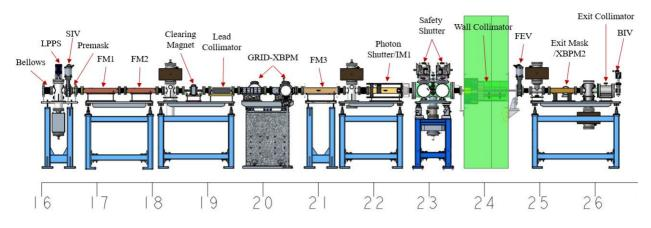
Figure 1: Layout of the HHLFE for APS MBA upgrade.
