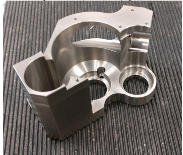
Figure 5: Main magnet mounting part.
