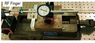
Figure 10: Test setup for cyclic fatigue testing of the RF fingers.
