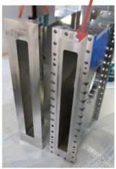
Figure 2: Left side BPMS as pre-part and on right a "ready part" of OTRS chamber with integrated "sealing grove", see arrow. (Photo taken by D. Nölle, DESY, Hamburg).
