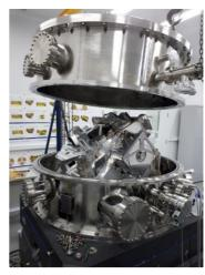
Figure 1: Overall view of the HD-DCM with its major subparts, namely: granite bench, double-side goniometric system, goniometer frame, long-stroke frame, 1st and 2nd modules, and the vacuum vessel. (For references, see [5].)
