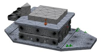
Figure 12: FE model of complete flexure stage. The orange arrow in the center is the gravity force, the red arrow an applied displacement, and the green arrows the fixed points.
