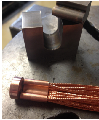
(a) Photo of the pressed braid-end and the pressing tool
