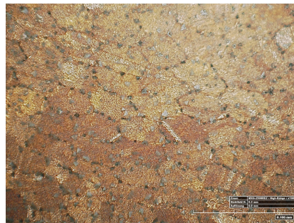
(b) Detail of the single wires, which have been deformed to hexagons. The single wires have a diameter of 0.05 mm.
