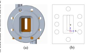
Figure 1: (a) CAD model of the mask assembly, front view; (b) CAD drawing of the mask model used in the analysis, front view, showing the beam footprint.
