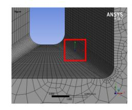
Figure 4: The mesh of the taper corner.
