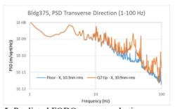
Figure 5: Predicted FODO magnet pole tip response using random vibration analysis. Blue is floor (input) while orange is magnet (response).
