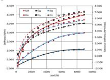
Figure 3: Airloc 2012-KSKCV translational (Kxx, Kyy, Kzz) and torsional (Ktx, Kty, Ktz) stiffnesses.
