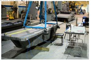
Figure 1: The FODO prototype girder casting at the manufacturer, rigged for a free BC EMA.
