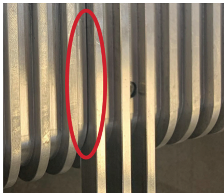
Figure 6: Interface where footed pole meets the magnet core where the conductor could potentially get pinched.
