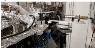
Figure 1: Autocollimator was aligned to us/in mirror at 2-ID prior to addition of reference mirror.
