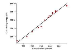
Figure 5: In situ autocollimator data from 4-ID-C SGM correlated with XPS measurements.
