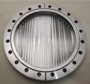
Figure 2: The vacuum vessel for the zero-length CF fintype NEG pump before oxygen-free Pd/Ti deposition.
