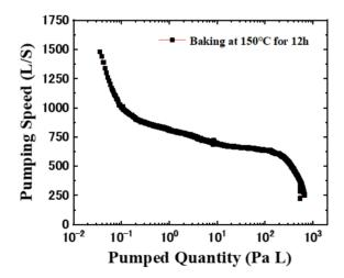
Figure 6: Pumping speeds of the zero-length CF fin-type NEG pump for H<sub>2</sub> after baking at 150 °C for 12 h, when the H<sub>2</sub> introduction pressure was  $1 \times 10^{-4}$  Pa.
