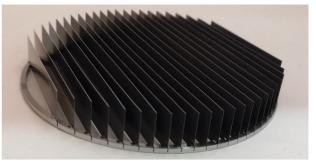
Figure 3: Ring with fins for the zero-length CF fin-type NEG pump before deposition of oxygen-free Pd/Ti. Reproduced from Ref. 19, with the permission of the Particle Accelerator Society of Japan (PASJ).
