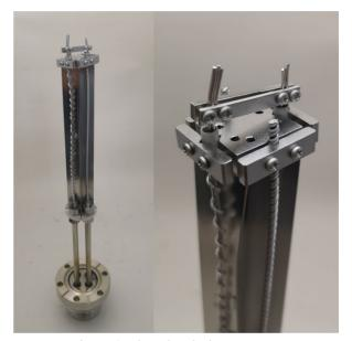
Figure 4: The Pd and Ti evaporator.
