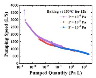
Figure 5: Pumping speeds of the zero-length CF fin-type NEG pump in various introduction pressures (P) of H<sub>2</sub> after baking at 150 °C for 12 hours. Reproduced from Ref. 19, with the permission of the PASJ.
