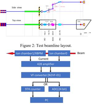
Figure 3: Data acquisition equipment.
