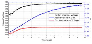
Figure 6: Cu K edge flux and absorption ratio for 9 hours.
