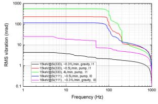
Figure 9: Integrated RMS displacement.
