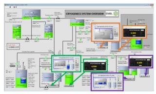
Figure 5: Cryogenics supervision system with access to sub-systems.
