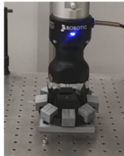
Figure 4: Sample wheel with Robot Gripper interacting 8-ID Lab test area.
